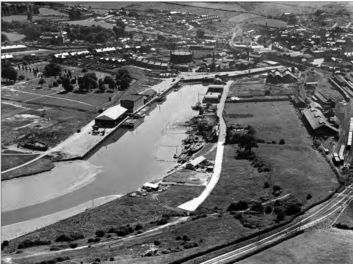
Figure 11 – The head of the Medina estuary in 1932, seen from the north. The layout of quays is largely the result of work in the 1850s. The gasometer of the gasworks is visible above centre. Little London lies to the west (right) of the estuary and sheds and sidings of the railway are visible far right, though the station lay just outside the frame. (EPW039658, © Historic England Archive - Aerofilms collection)
