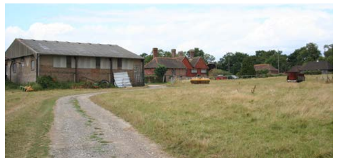
This large, dispersed multi-yard farmstead has several detached yards including two large, covered yard buildings; the large shed in the foreground formerly had a series of gabled roofs that have been replaced and raised. Additionally, many of the buildings are ranged alongside a track that runs through the farmstead, giving this group a dispersed, driftway character. Photo © Bob Edwards
