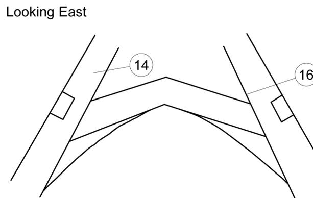
Figure 10: Sketch showing the location of samples SWM-F14 and SWM-F16 from truss B in the hall range roof
