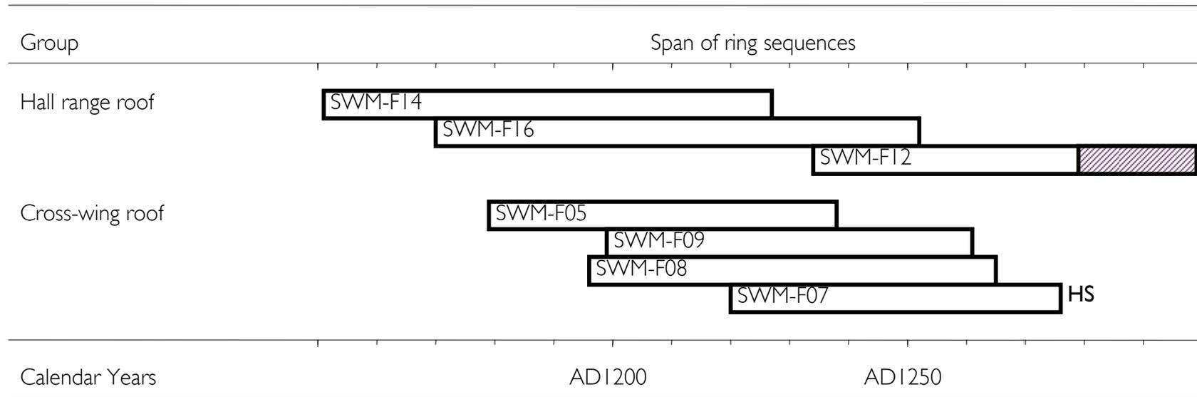
Figure 12: Bar diagram of samples in site chronology SWMFSQ01 and the individually dated sample SWM-F12. White bar = heartwood rings; hatched bar = sapwood rings; HS = the last ring of the sample is at the heartwood/sapwood boundary
