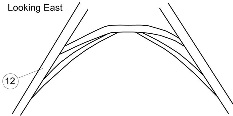
Figure 9: Sketch showing the location of sample SWM-F12 from truss A in the hall range roof
