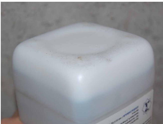
Figure 9 Inverted bottle of nanolime showing how, after storage, particles settle at the bottom of the bottle. If allowed to accumulate for too long, particles will agglomerate and shaking will not fully separate them.
