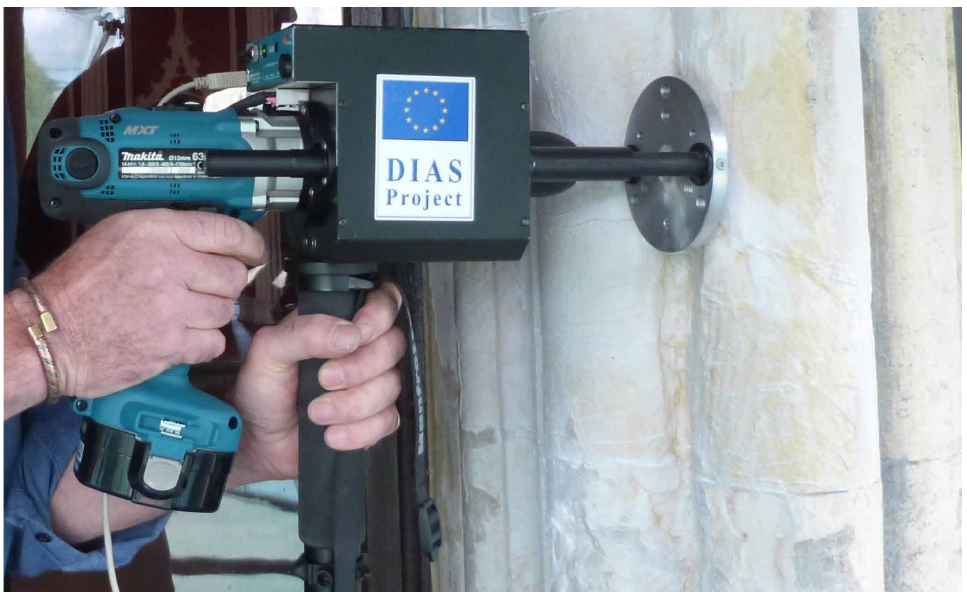
Figure 32 Using the Drilling Resistance Measurement System (DRMS).
