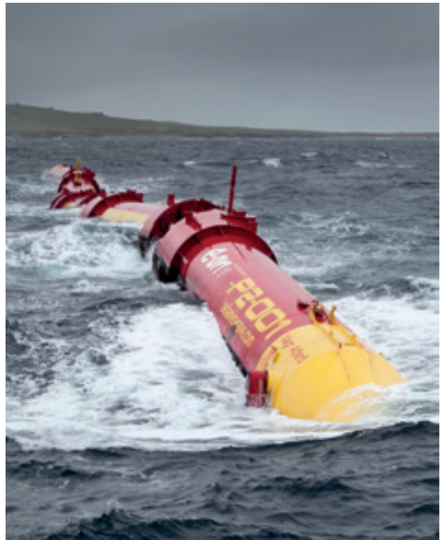
The Pelamis is a wave device that floats on the surface and is tethered to the seabed. It is designed to operate in relatively deep water offshore. Image © Pelamis Wave Power.
