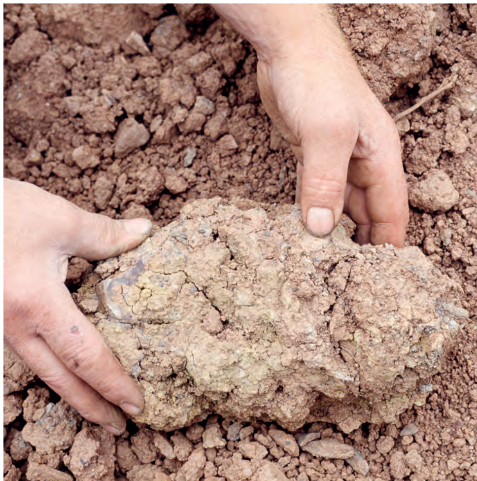
For repairs to cob walls at Bowhill, near Exeter, subsoil was obtained from a nearby excavation for a reservoir.
