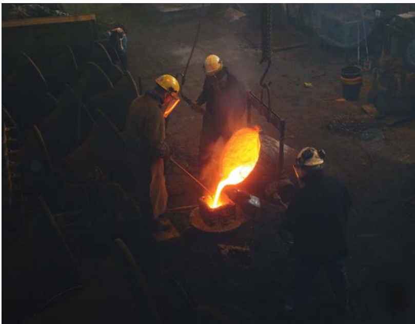
Taylor's Foundry, Loughborough. One of only four bell foundries surviving in Europe and one of two in England. Bells are cast in the medieval manner, in the floor of the foundry.
