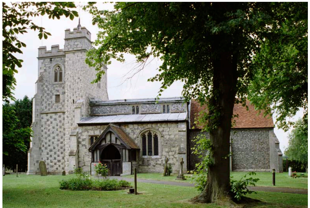
Figure 7: St Mary's Church, Puttenham. Knapped flint and Ketton Stone chequerwork.
