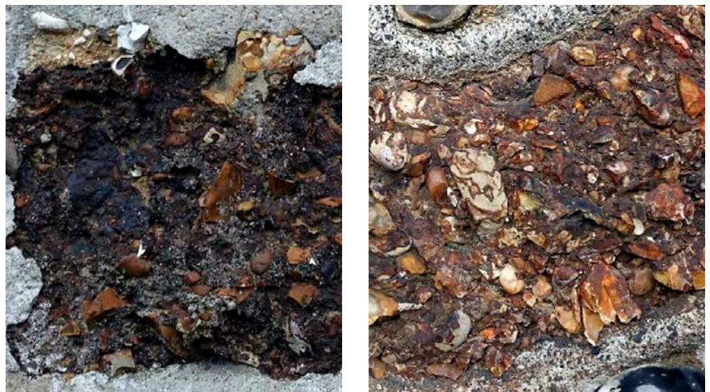
Figure 45: Wingrave Puddingstone (left); Iver Puddingstone (right).
