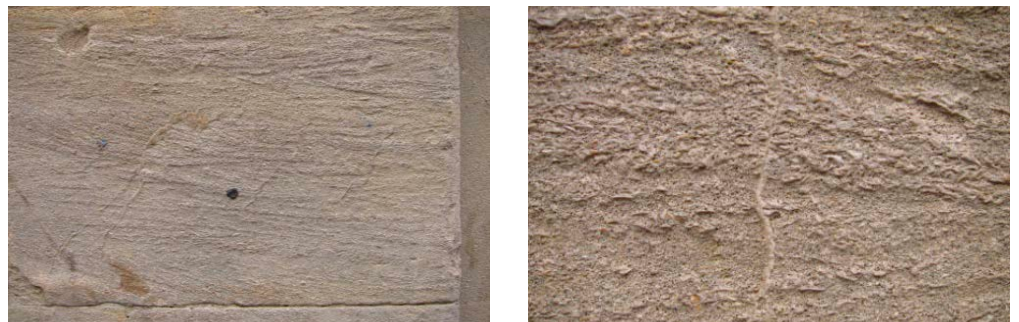
Figure 26: Combe Down Stone details showing fine-grained shell debris and calcite-cemented stringers.
