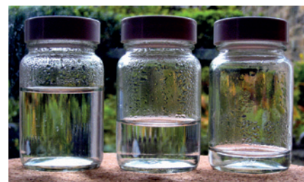
The air inside all three sealed bottles is saturated (as shown by the condensation) and this is independent of the water level. There are more than a 'vigintillion' (10 20 ) water molecules in a single drop of water, so the reservoir needed to reach saturation is tiny.
