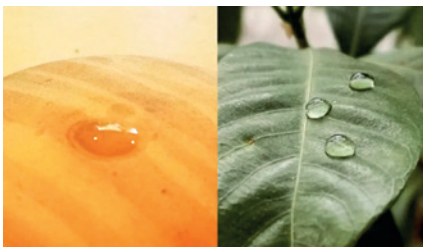
Water will interact strongly with most surfaces. Left, a droplet of water on a surface that is 'hydrophilic' ('water-loving', so reacting with water molecules); right, a droplet on a 'hydrophobic' surface.
