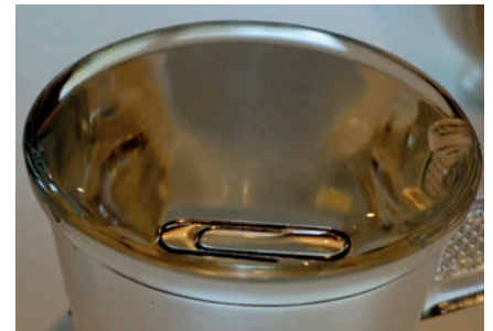
The structure of water molecules allows them to cling together strongly, forming a strong ‘meniscus’.
