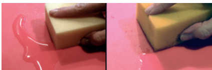
For the same reason that a sponge must be slightly wet if it is to soak up a spill, dry building materials resist absorbing water. On the other hand, wet materials will draw water in quickly: the 'moisture history' of the material is therefore of paramount importance.
